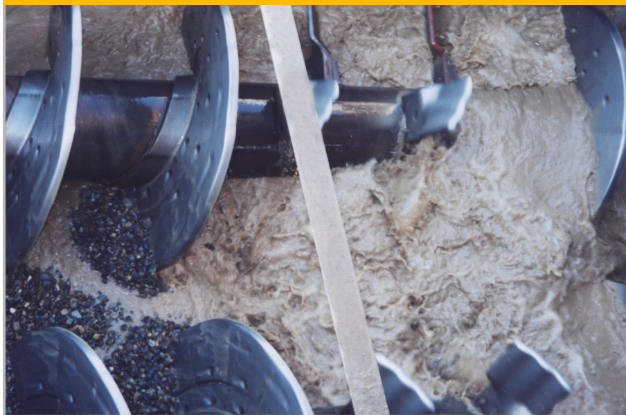
A look inside at the paddles and shaft of a coarse material screw washer.
